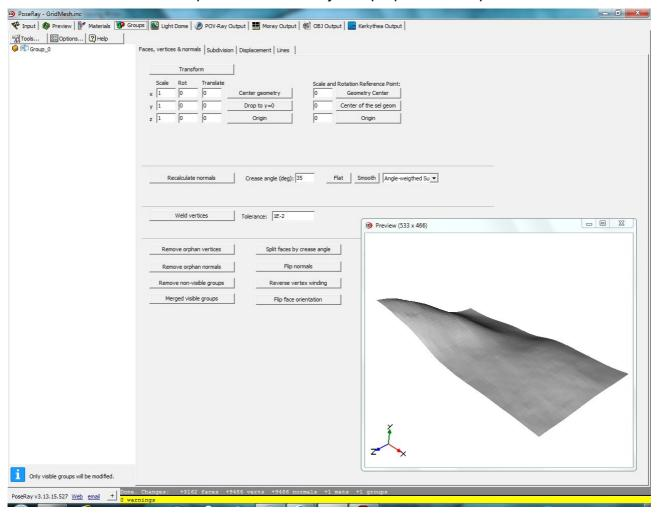
In the Groups tab of Poseray, the only necessary action is to apply "Weld Vertices" as the individual triangles in the original mesh{} are not bound together:
